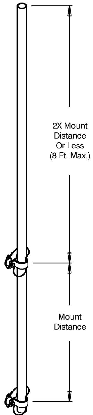
**In all cases the system should be mounted as solidly as possible to the most rigid part of the structure.**
