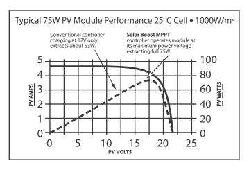
The actual charge current increase you will see varies primarily with module temperature and battery voltage. In comfortable temperatures, current increase typically varies between 10 to 25%, with 30% or more easily achieved with a discharged battery and cooler temperatures. What you can be sure of is that Solar Boost charge controllers will deliver the highest charge current possible for a given set of operating conditions.
