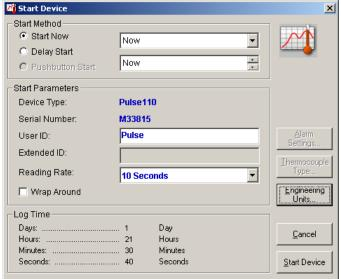
If a 10 second reading rate is acceptable, click the "Start Device" menu bar option to start the device. Wait for a dialog box to appear that indicates the device has been started successfully. Unplug the interface cable, and replace the stainless steel watertight plug.
