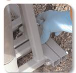
Fasten 2 remaining bolts to secure base in upright position.
