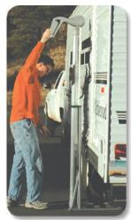
Install nested telescoping tower & AirX wind generator onto base support.
